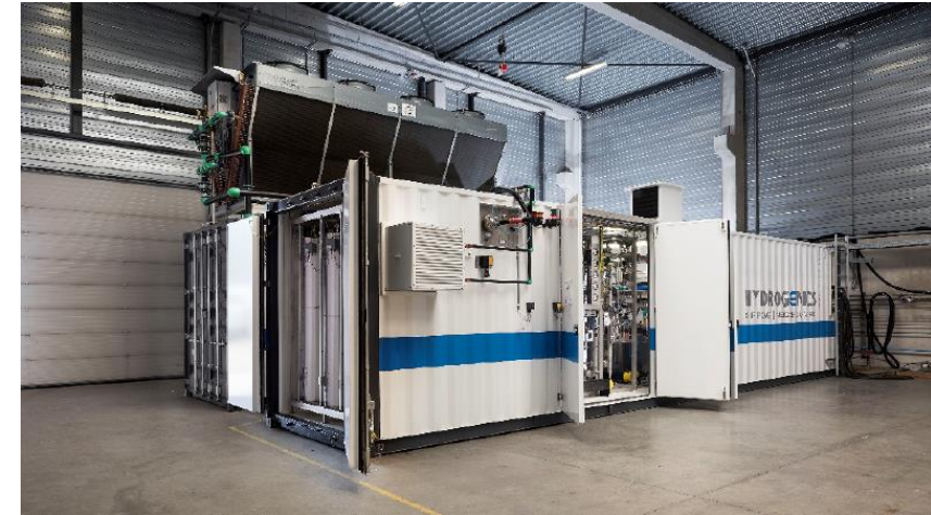
An example of an electrolyser HyLYZER 500-30 bar
